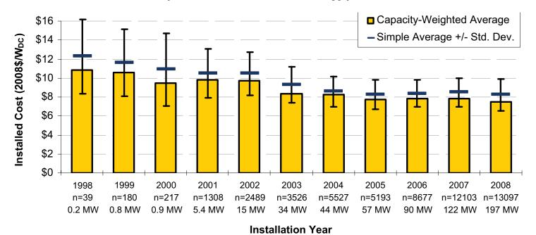
Figure 2: Falling installed cost for solar PV, 1998–2008 (Wiser, 2009).
