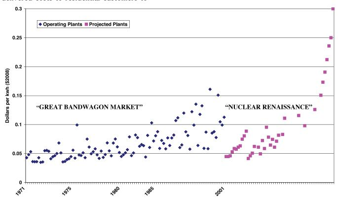
Figure 4: Nuclear power generation cost — operating reactors compared to proposed reactors (Cooper, 2009).
