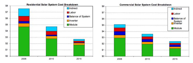
Figure 3: Residential and Commercial cost breakdown for solar PV in 2005 \$ per watt installed, 2006–2015, U.S. Department of Energy.8
