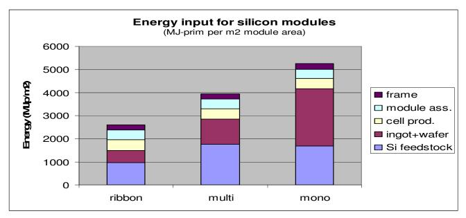
Figure 3: Energy input for crystalline silicon modules, in MJ of primary energy per m<sup>2</sup> of module area, with the contributions of consecutive process steps.
