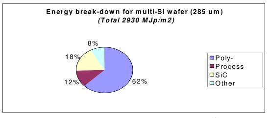
Figure 4: Energy input breakdown by source for a multi-Si wafer (125x125 cm<sup>2</sup>, 285 um thick)
