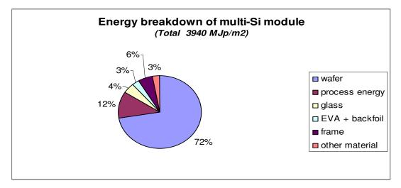
Figure 5: Energy input breakdown by source for a multi-Si module (72 cells, 165 Wp). Note that production of 1 m<sup>2</sup> of module area uses only 0.92 m<sup>2</sup> of wafer area as input.
